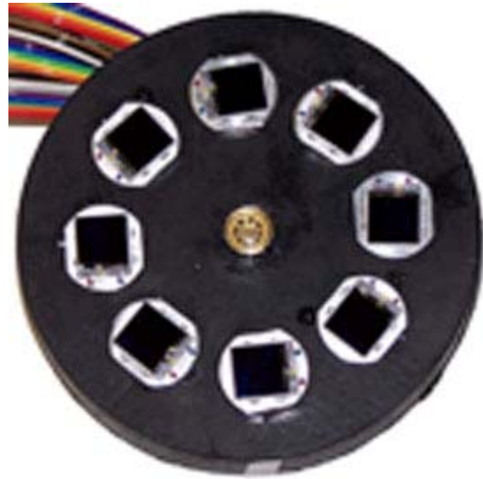
(b) 1 sources 2 detectors system based on our LED imager
